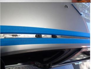
Apply protective tape as shown in the image and place the rubber packer on the vehicle roof first, and then loosely fit the mount bracket.
