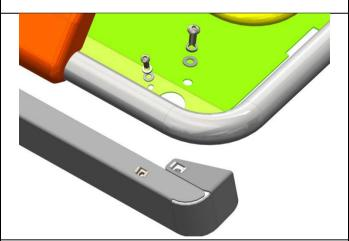
Fit 3 x M6 and 2 x M8 cage nuts to air deflector as shown. Secure to rack using M6 button head screw, M6 spring and flat washers, M8 button head screws, M8 spring washers and flat washers.
