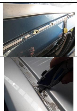
1. Unclip the exterior roof trim from both sides of the vehicle. Take care not to bend the trim, as it will be reused.
