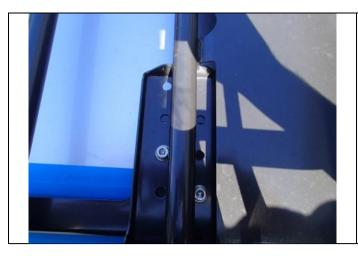
14. Fix the roof rack in place using eight M8 x 30mm socket head cap screws, M8 flat washers, M8 spring washers and four bolt plates. Centre rack and tighten all bolts to their specified torque.
